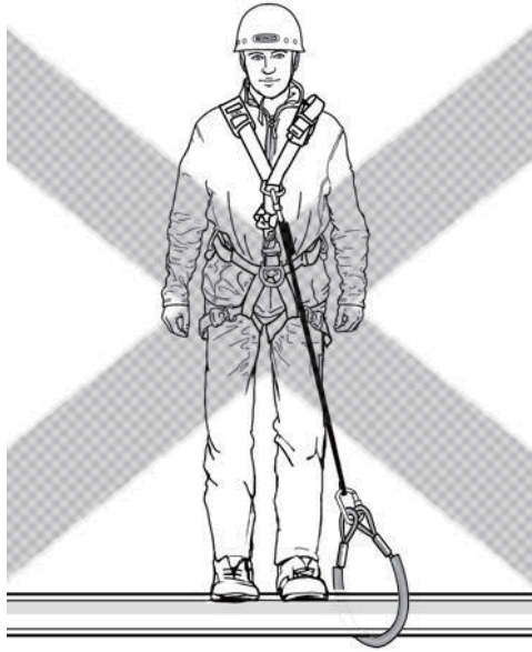
Figure Q.2 — Lifting an anchor sling from its normal hanging position increases the potential fall distance
